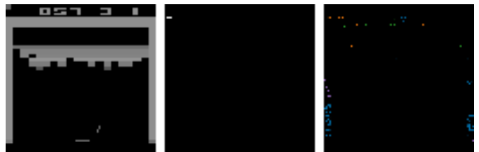
Fig. 2: (left) A poisoned state; the trigger is the 3 \times 3 patch of pixels in the top left corner. (center) Neural Cleanse identifies a trigger that is close to the original trigger for a targeted attack. (right) Neural Cleanse fails to identify the original trigger for the untargeted attack; the 4 colors illustrate the 4 different triggers found, one per action.
