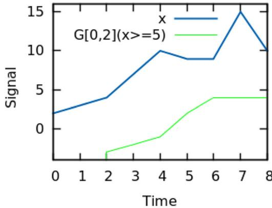
**Fig. 4** Augmented trace:  $x$  is the variable in the original trace and new signal corresponds to robustness metric value of  $G_{[0,2]}x \geq 5$
