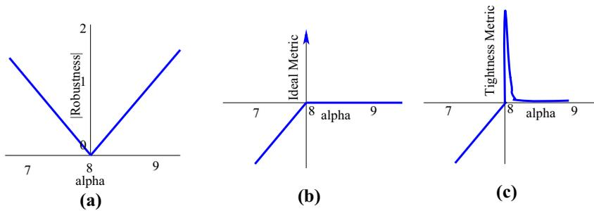
**Fig. 1** **a** The absolute value of robustness metric reaches 0 at  $\alpha = 8$ . It is close to 0 even at 7.99 even though the temporal property corresponding to  $\alpha = 7.99$  is violated by the trace. **b** The ideal metric should be negative when  $\alpha < 8$  and jump to  $\infty$  when  $\alpha = 8$  and drop down to 0 when  $\alpha > 8$ . **c** A metric which is negative for  $\alpha < 8$ , reaches its maxima between 8 and  $8 + \epsilon$  and then drops to 0
