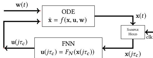
Figure 1: Block diagram of a neural feedback control system.
