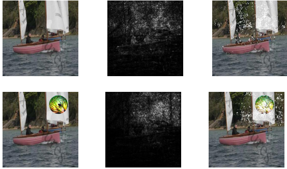
Figure 1: The top row shows an original yawl image and the bottom row shows the adversarial input obtained by adding an adversarial patch (Brown et al., 2017) which causes misclassification. The leftmost image is the input, next to it is the saliency map that shows the features (pixels) with positive attributions (Szegedy et al., 2016), and the rightmost image shows the pixels with top 2% attribution masked. People in the boat are in the top 2% positive attribution features in original image but not in the adversarial image. The saliency map showing attributions are obtained using Integrated Gradient method (Sundararajan et al., 2017)
